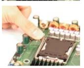
2. Gently lift the socket clip to open the load plate.
